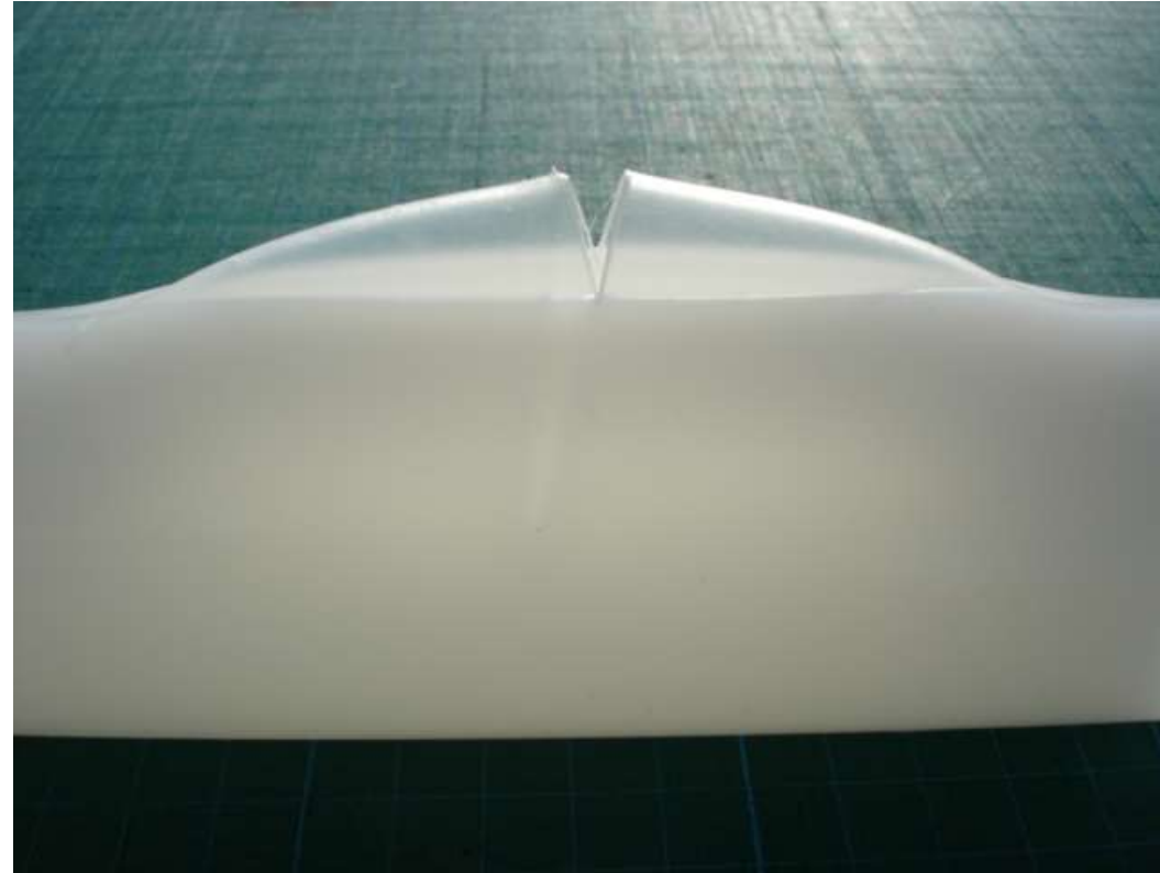
Rotomoulded pipe after long exposure to stress exhibiting ductile (bulging) failure
